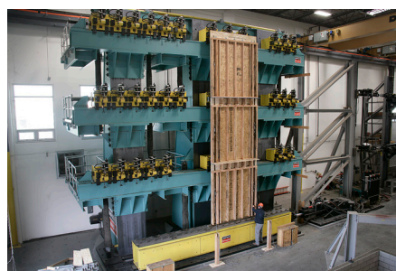
Test of a full-size three-storey building. Simpson Strong-Tie - Tyrel Gilb Laboratory in Stockton
