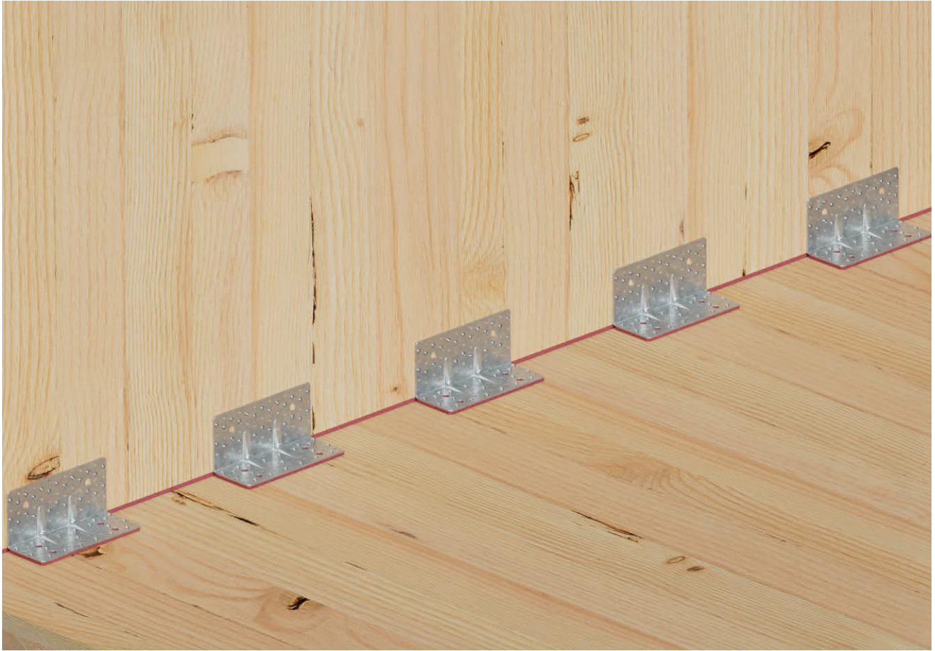
CLT Wall to CLT Floor
