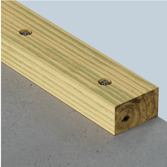
CLT Wall to Concrete
