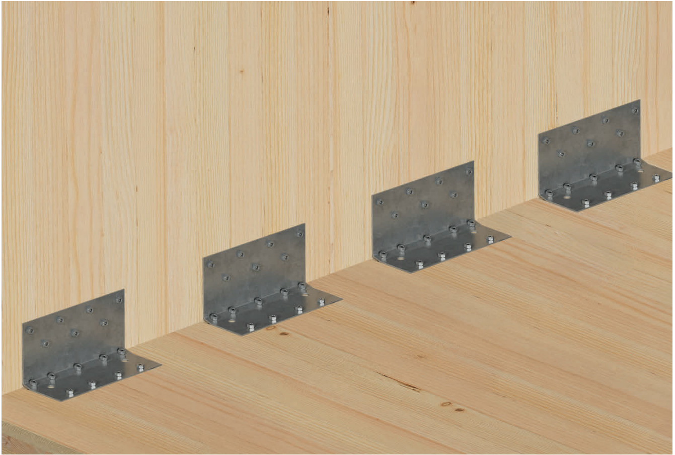
CLT Wall to CLT Floor
