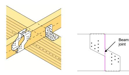
Conditions for using I-beam joists.
